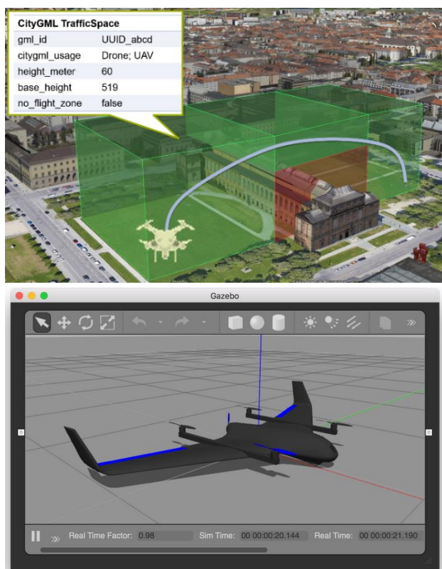
3D city model including 3D air spaces representing potential drone flight zones and drone model in Gazebo
